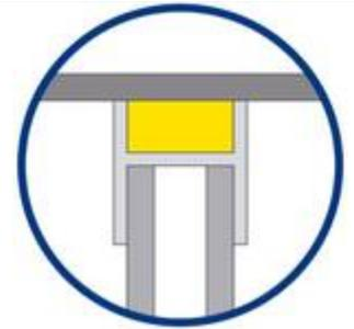
Where an 'H' section is used at the partition head, this should be infilled with the appropriate grade.
