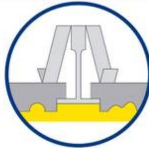
For rebated edge tiles with a deep profile pattern an increased thickness should be used. A cut piece is inserted separately into the rebate.
