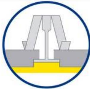
For rebated edge tiles with a flat or small surface pattern, the minimum thickness can be used. A cut piece is inserted separately into the rebate.
